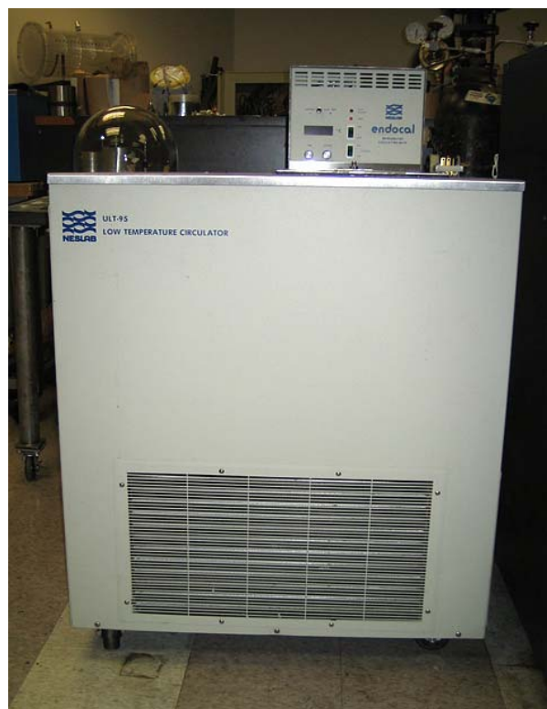
Figure 13 Hot water heater (top) and low temperature circulator (bottom).
