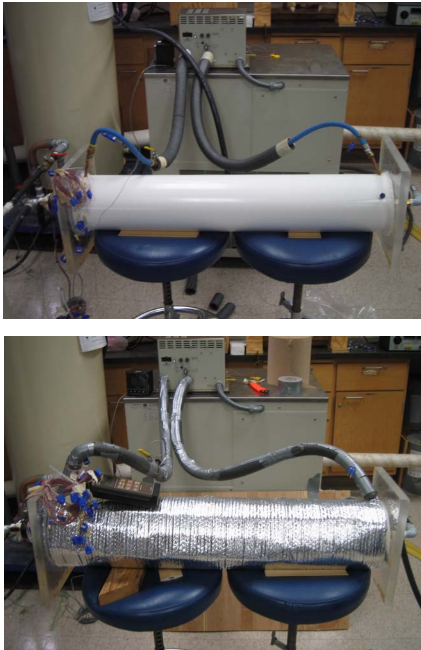
Figure 12 Before(top) and after(bottom) application of insulation.
