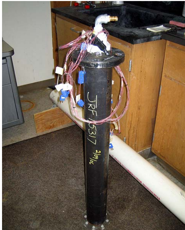
Figure 9 Prototype pipe with thermo couples.
