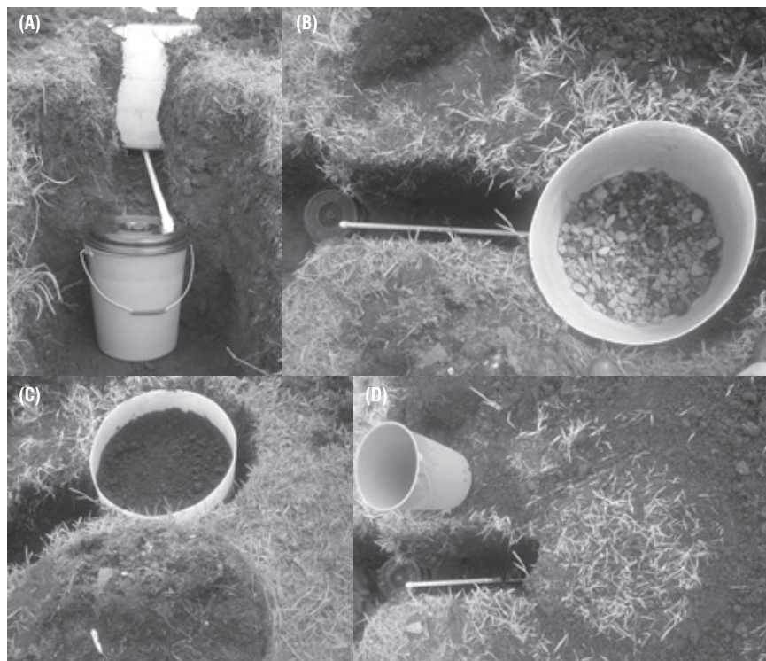
FIGURE 1. (A) Cross section of the drainage lysimeter. (B) Top view of the drainage system 0.1 m of fine gravel + 0.1 m of large gravel. (C) Lysimeter with the soil layers stockpiled. (D) Lysimeter with the grass cover.
