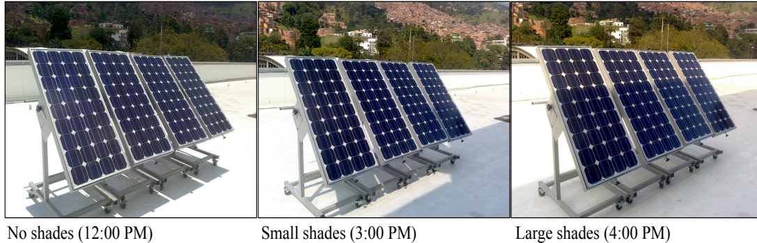
Figure 3-21.: PV array in series-parallel structure.
