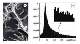
Figure 2-9.: (a) Fractogram of a typical ductile fracture of bridges between fragments of brittle cleavage fracture in neighboring areas of the fracture (b) and brightness histogram of this image. [66].
