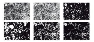
Figure 2-11.: Successive transformation of an input fractographic image (a), Segmented images as result of pixel fragmentation inside five subsets (b), with isolation of typical elements (c), dimples formed (d), bridges formed between them (e), and edge dimples conglomeration (f) [66].
