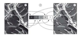
Figure 2-10.: Scheme of a fractographic image conversion (a) using shine levels as labels (b) Inside a segmented image (c) [66].
