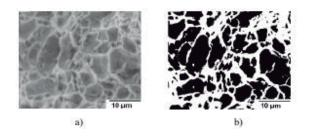
Figure 2-13.: Fractography of a metal welding; Original image (a) and segmented image (b) [17].
