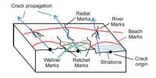
Figure 2-5.: Common marks that can be find on fracture surface of mechanical elements[34].
