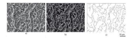
Figure 2-14.: Fiber extraction in a fatigue fracture surface image; (a) normalized image (400 X 300 pixels), (b) fiber detection, (c) significant fiber traces [73].
