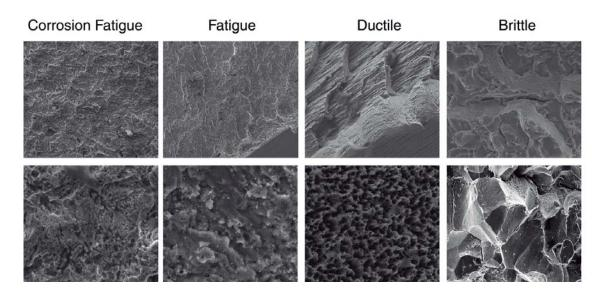
Figure 5-2.: Samples of SEM images from the fracture database used in this paper.
