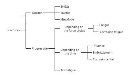
Figure 2-4.: General classification of more common fracture failure modes in metallic materials, according to its sudden or progressive nature [34]. The fractures to work with are framed in a square.
