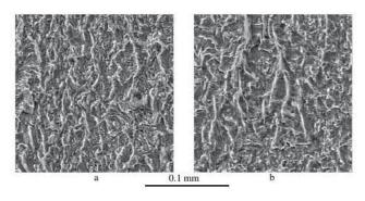
Figure 2-6.: Samples of typical texture on a fatigue fracture surface. Low (a) and High (b) CGR. AISI304L stainless steel [72].
