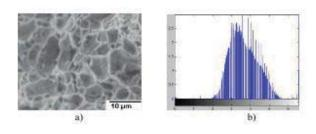
Figure 2-12.: Fractograppy of a metal welding (a) and the image histogram (b) [17].
