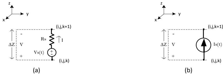
Figure 4 Source Modeling into the Yee's Cell (a) Lumped Voltage Source with non-zero internal impedance (b) Current Source
