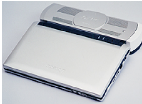
Fig. 24. Toshiba's DMFC for a laptop
