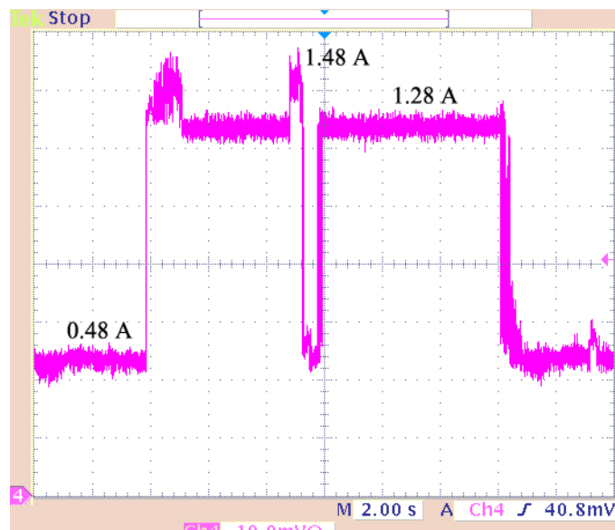
Fig. 34. Load current of Dell Latitude C600 during the saving of a MS Word document
