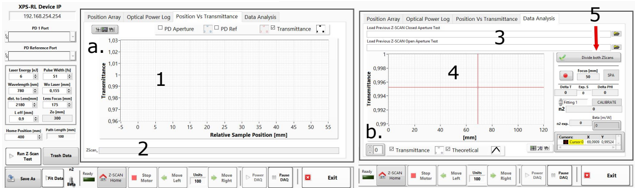
Figure 4-4.: Z-scan tab software implementation. (a) 1. Data plot in real time. 2. File path. (b) Data analysis tab: extraction of n_2 and \beta as well as laser variables tuning
