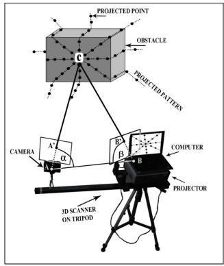
Figure 1. Stereovision principle used in the proposed 3D scanner
