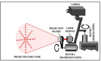
Figure 5. Laser based measurement system
