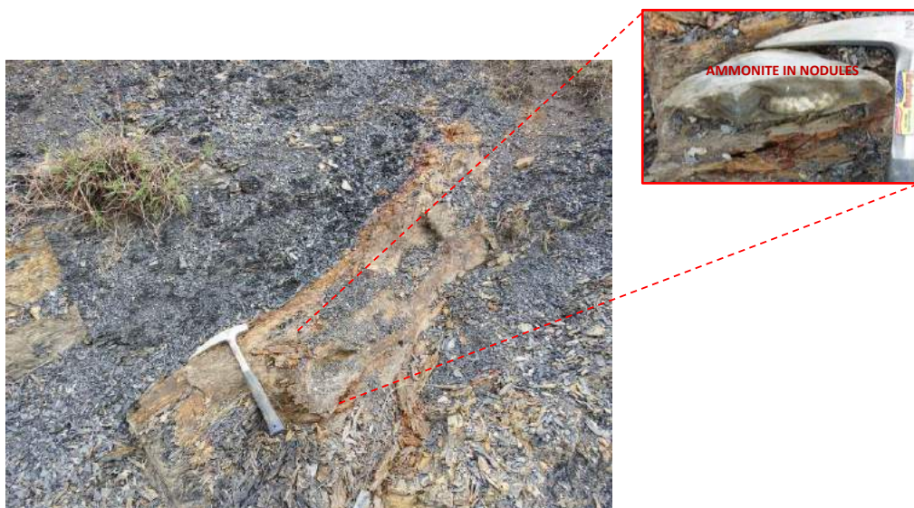
Photo 3.9. Showing the characteristic lithology from La Paja Formation with black to gray shales and a red level of claystones with nodels, sometimes with ammonites (right upper square).
