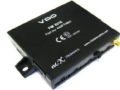
The FM 3316 on-board computer interfaces directly with the vehicle's data bus supporting the CAN - J1939 and J1708 - J1587 standards.
