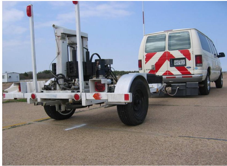
Fig. 35 One marked steel bar sensor under the center of load disk of FWD
