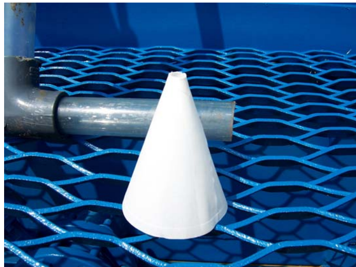
Fig. 67: Pipe for Sand Injection through Tank Outlet (Left) and Paper Cone for Pouring Sand into the Pipe (Right)
