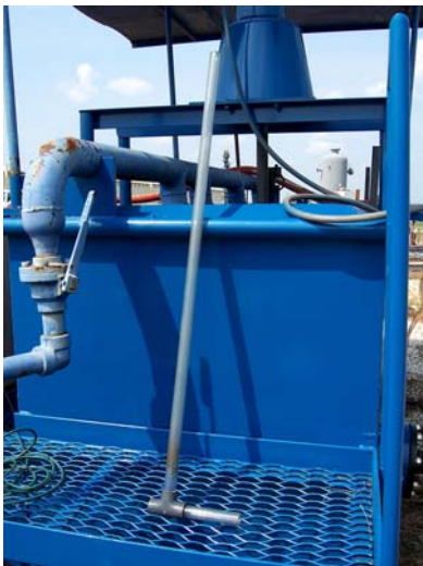
Fig. 67: Pipe for Sand Injection through Tank Outlet (Left) and Paper Cone for Pouring Sand into the Pipe (Right)
