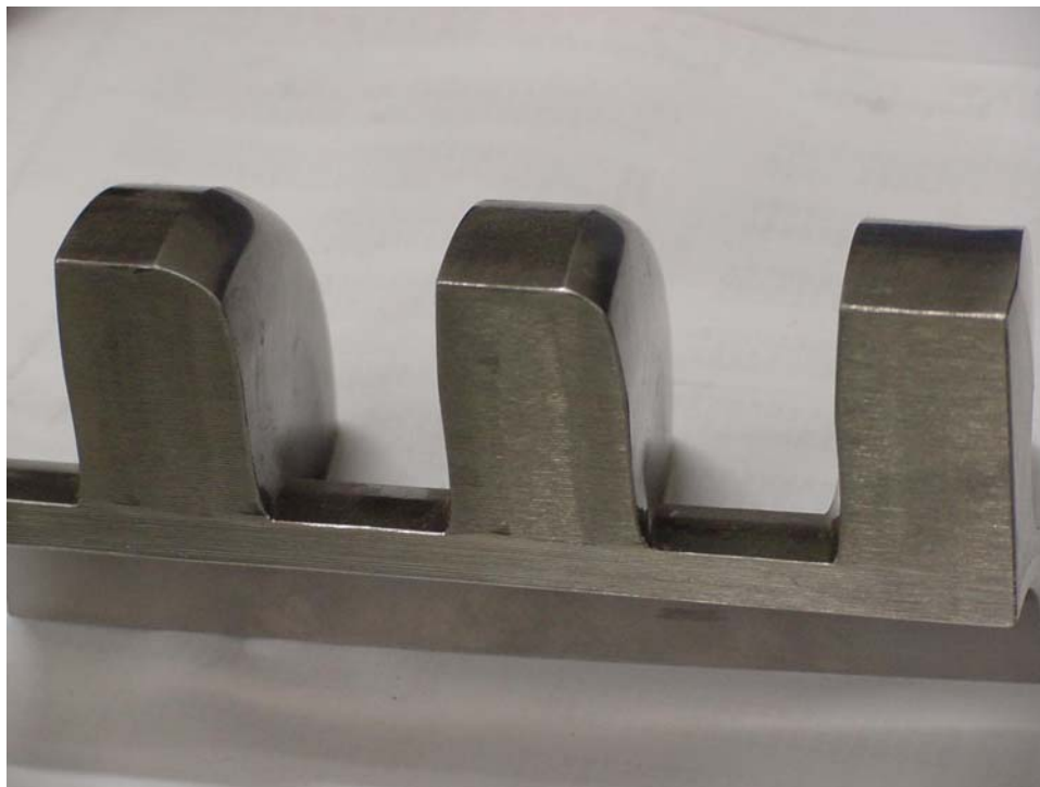
Fig. 82: Screw Erosion on Edge
