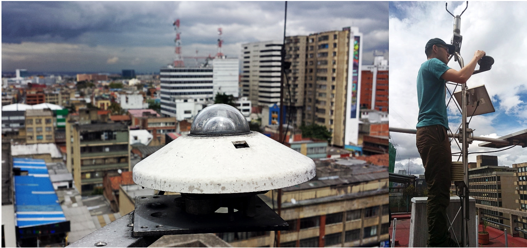
Figure 4-3.: Left: the pyranometer of the station “EL IDEAM”; Right: the author and the pyranometer.
