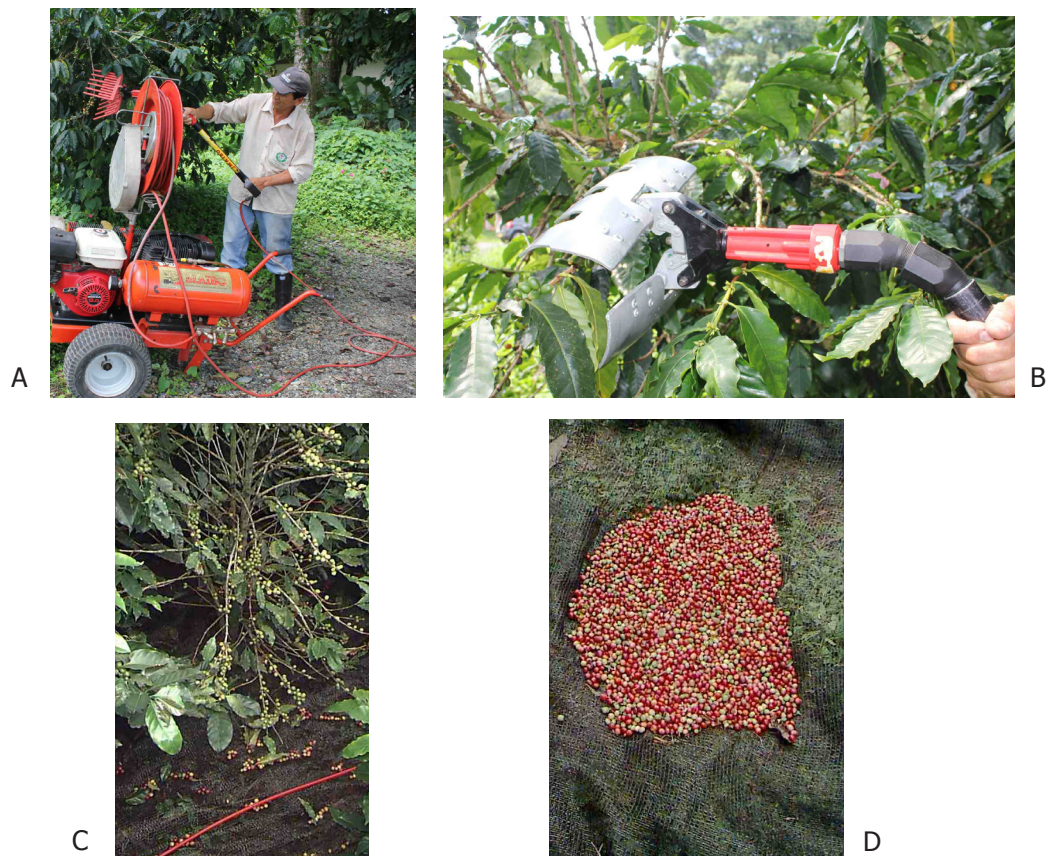
Figure 3. Personnel and equipment used to harvest coffee with a CENICAFE-I beater (A-B); state of the trees after sweeping with a CENICAFE-I beater (C) and harvest quality with a CENICAFE-I beater (D).
