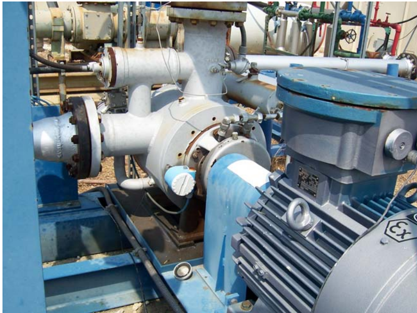
Fig. 4.1 – Bornemann MW-6.5zk-37 twin-screw pump with internal recirculation chamber.
