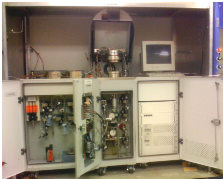
Figure 5 Overall view of APTAC system
