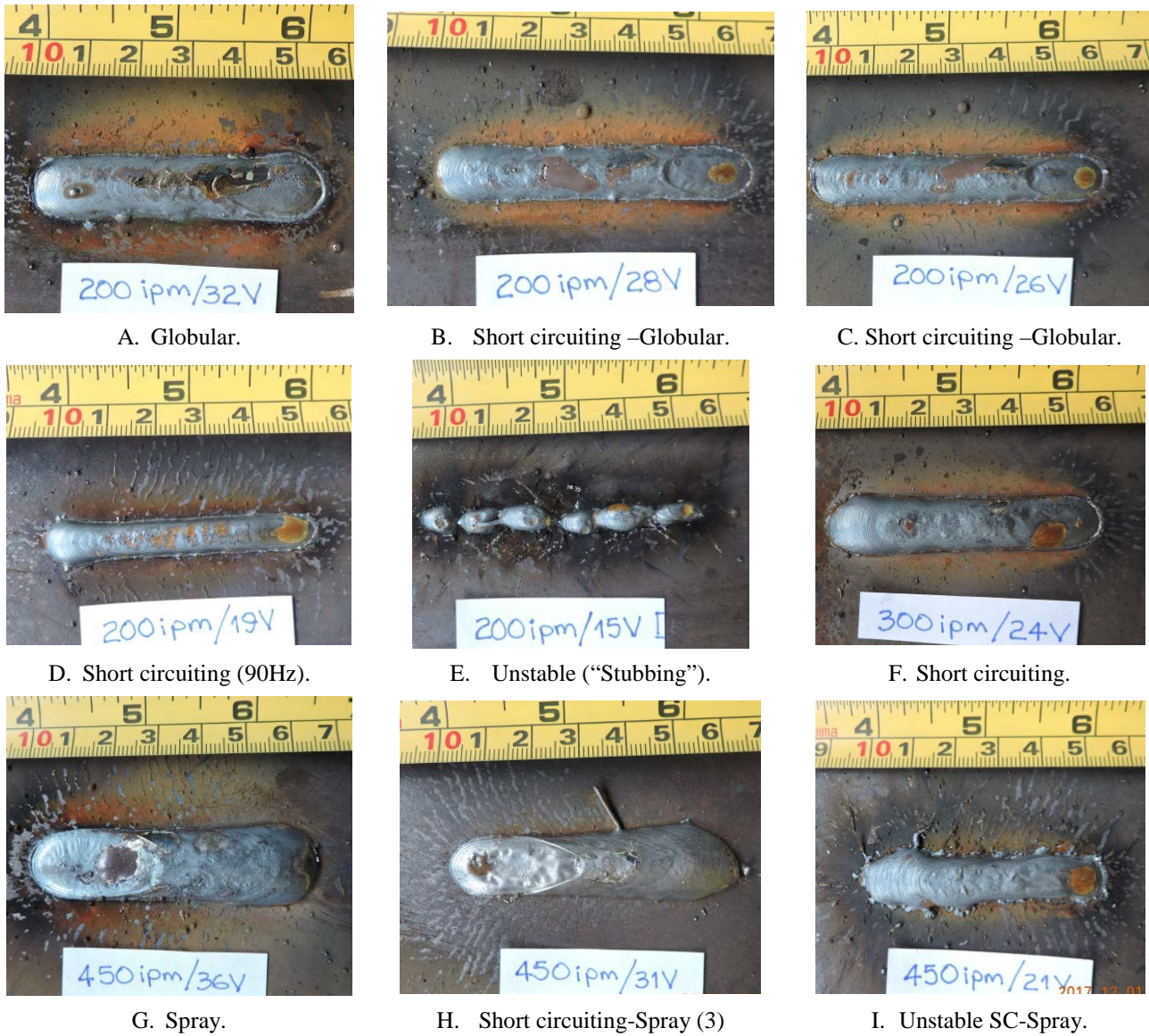
Figure 6. Weld bead's appearance obtained with several metal transfer modes. Source: Authors' own work.
