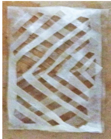
Figure 2.5. A) Chevron Geometry recommended for RED [41]. B) Spacers cut by hand used in the stacks.
