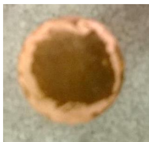
Figure 2.16. Oxidation reactions in copper stack terminals.
