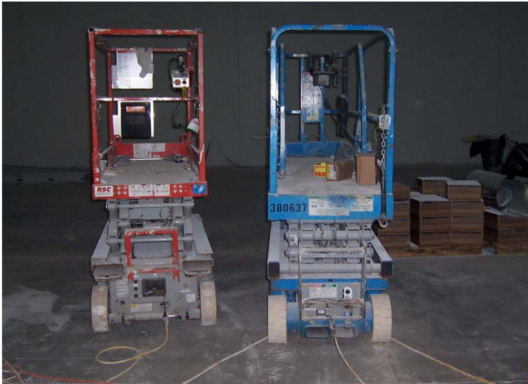
Figure 17. Charging Scissor Lift Batteries Overnight
