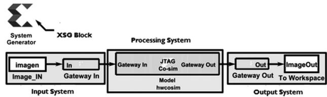
Figure 3. Implementation of co-simulation hardware (Xilinx, 2009).
