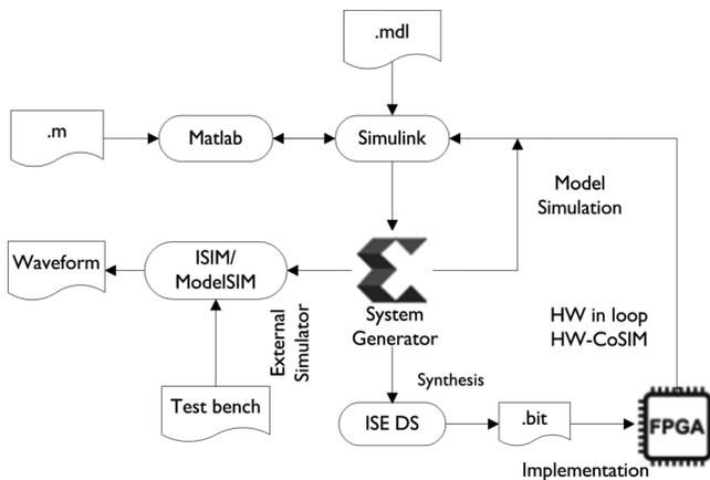
Figure 2. Project development flow with System Generator (Xilinx, 2009).
