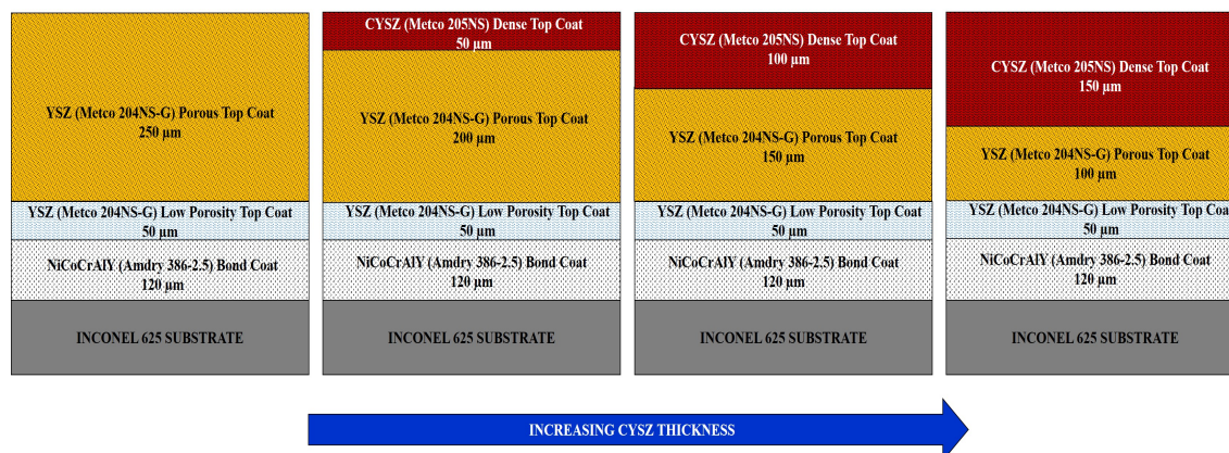
Figure 4.8: Experimental procedure to spray D-CYSZ/YSZ bilayers.
