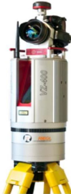
Figure 3-6 REIGL VZ-400 terrestrial scanner with the attached top mounted NIKON full frame camera used in this investigation
