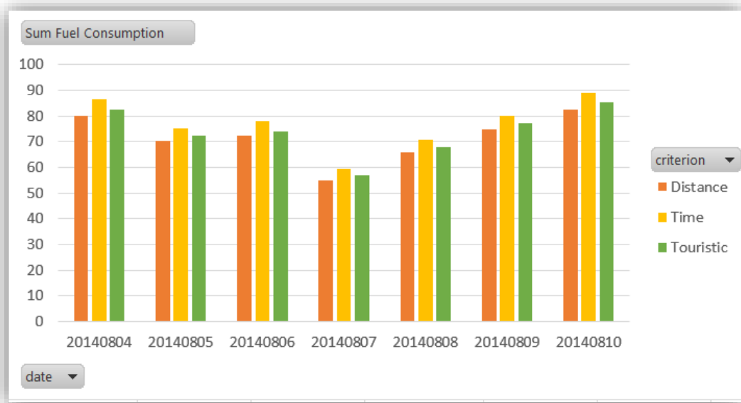
Figure 4.11. Fuel Consumption (litres / 100km) sliced by day and criteria
