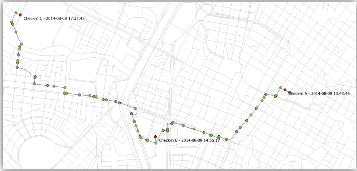
Figure 3.13. Reconstructed Trajectory using Distance Criteria from the user 1
