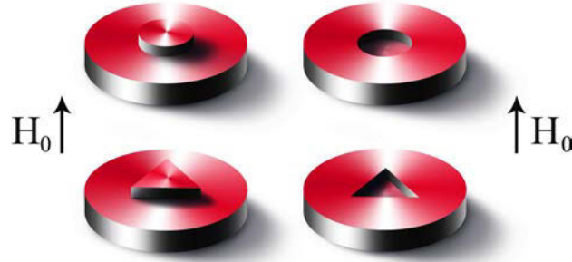
Figure 6-1: Layout of the studied sample: Superconducting disk with a central defect, hole (right) or barrier (left), for circular (up) or triangular (down) case. With a superconductor/vacuum interface.
