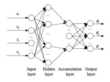
Figure 1. Schematic diagram of the multi-class classification PNN.
