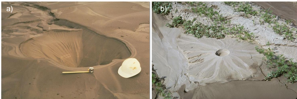
Fig. 1. Sand Boils generated after the earthquake: a) 1989 Loma Prieta earthquake, and b) 1979 Imperial Valley earthquake (after NISEE 2016).
