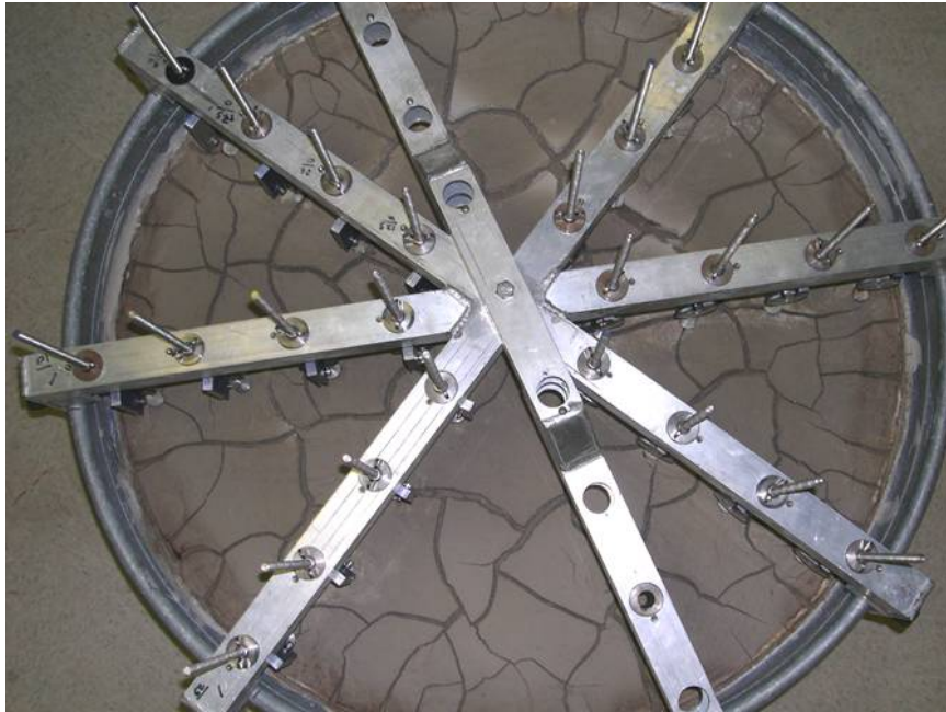
Fig. 4.26. Soil surface cracks after starting the first drying period.
