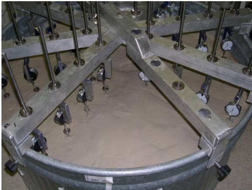
Fig. 4.22. Instrumentation of the large scale laboratory test tank.
