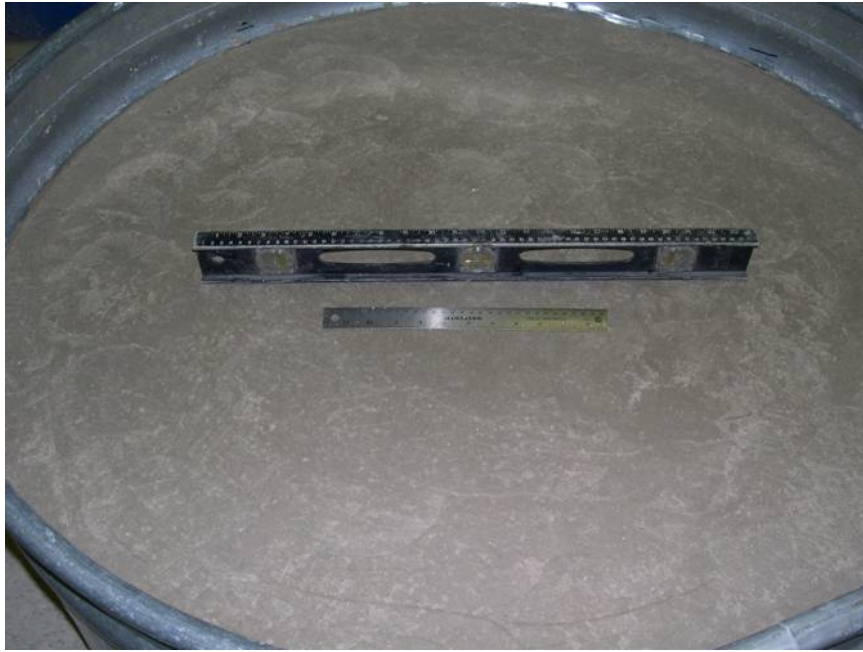
Fig. 4.21. Leveled soil surface after completing compaction.
