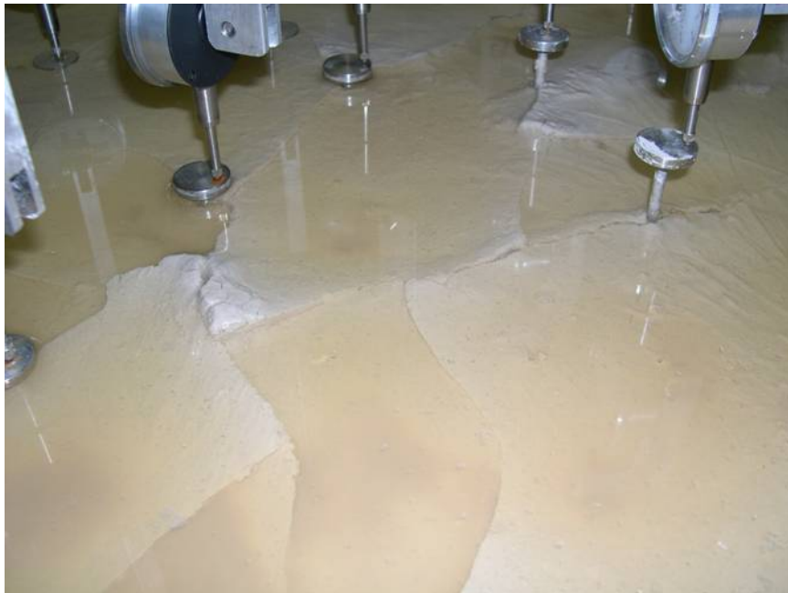
Fig. 4.27. Inundation to start the second swell cycle.
