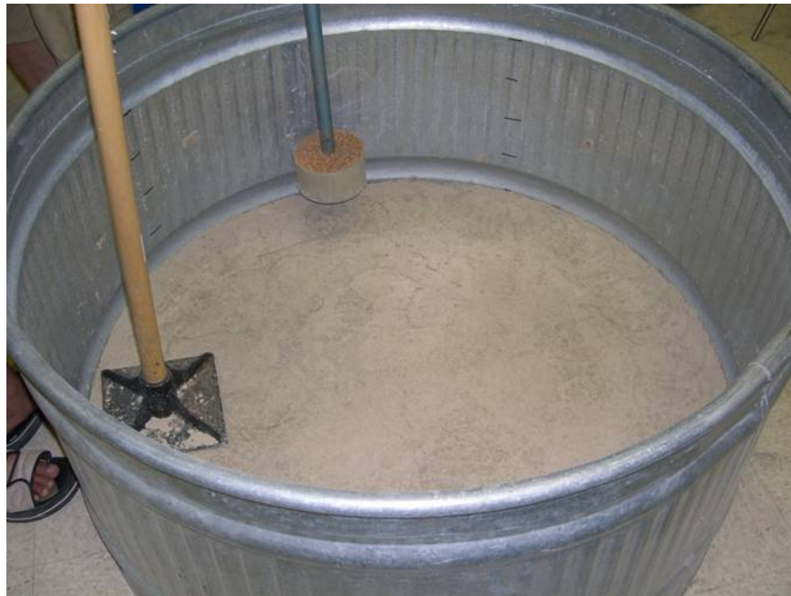
Fig. 4.20. Compaction of the clay soil in the tank.
