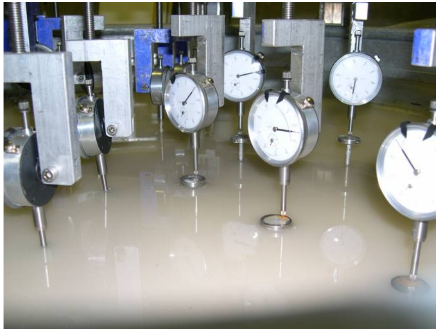
Fig.4.25. Inundation to start the first swell period.
