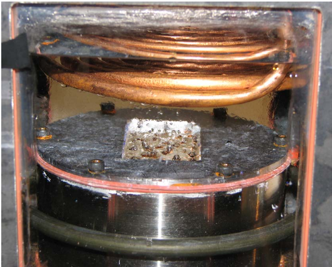
Fig. 19. Film boiling occurring at a subcooling level of 30 °C on a wafer coated with Type-A CNT.
