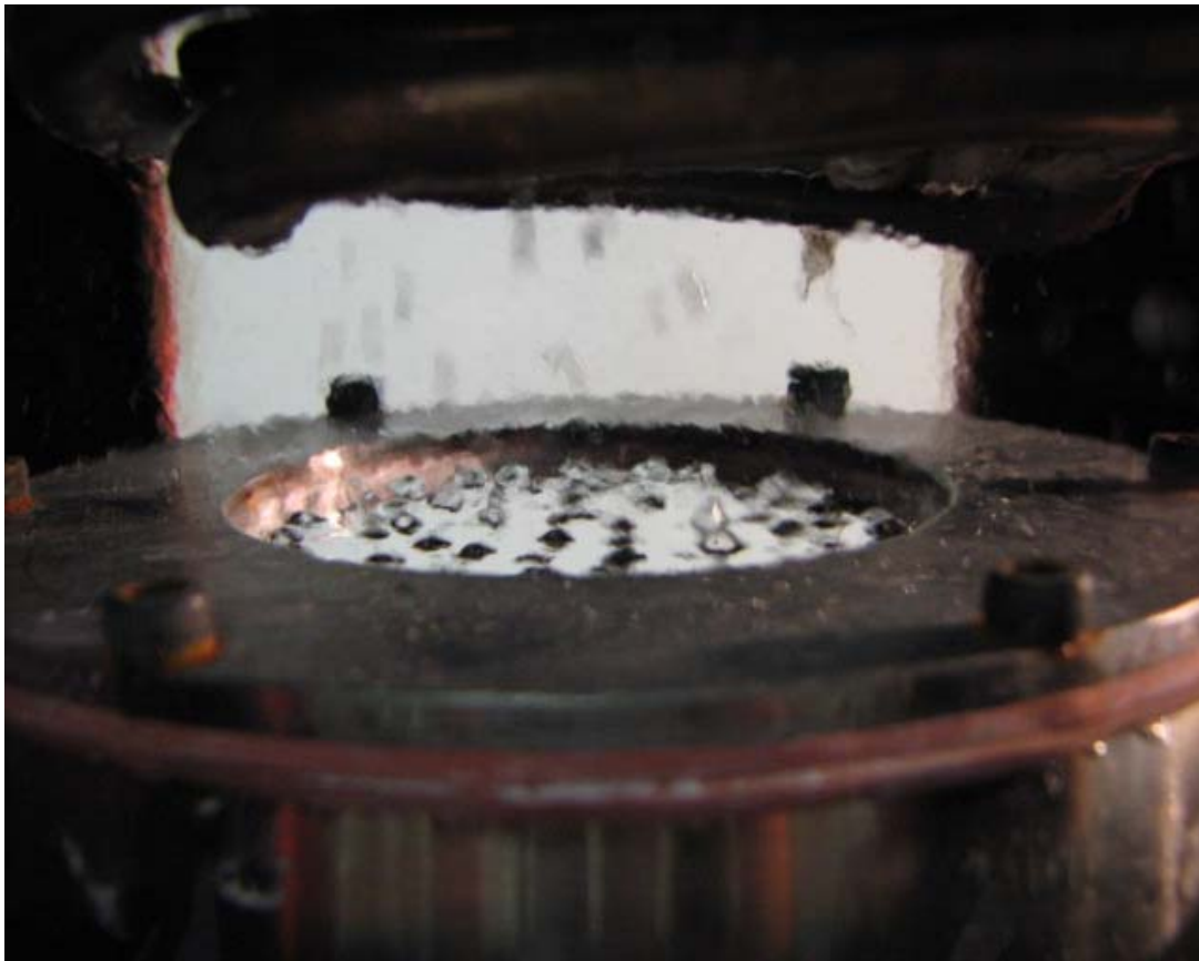
Fig. 18. Figure shows the non-departing bubble condition on a silicon wafer at \sim 37^\circ\text{C} subcooling level.
