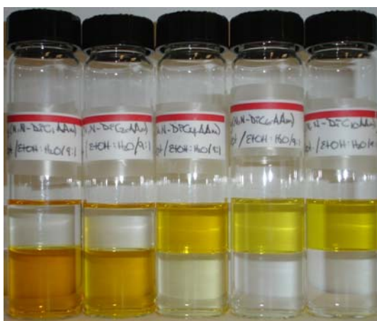
Figure 18. Heptane/90% EtOH-H 2 O biphasic systems for poly( N,N -dialkylacrylamide)s.
