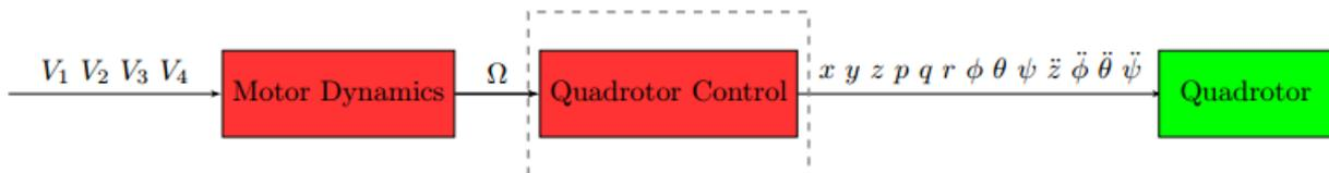
Figure 3.4: Control Diagram with voltage inputs
