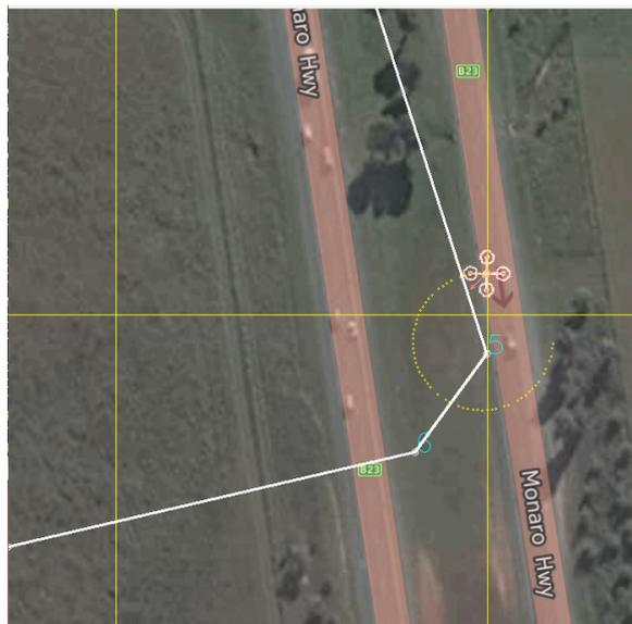
Figure 4.33: Application of Dubins Path with Waypoints in Auto/Circle Mode 1
