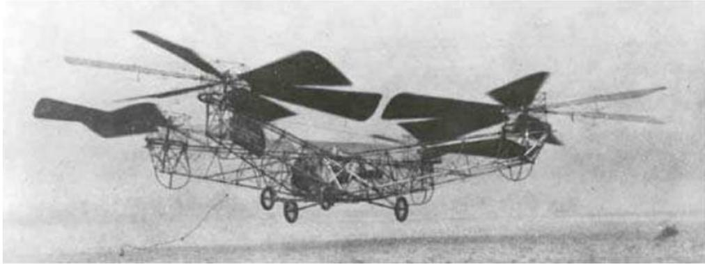
**Figure 1.11:** *Quadrotor built by Georges de Bothezat and Ivan Jerome*
