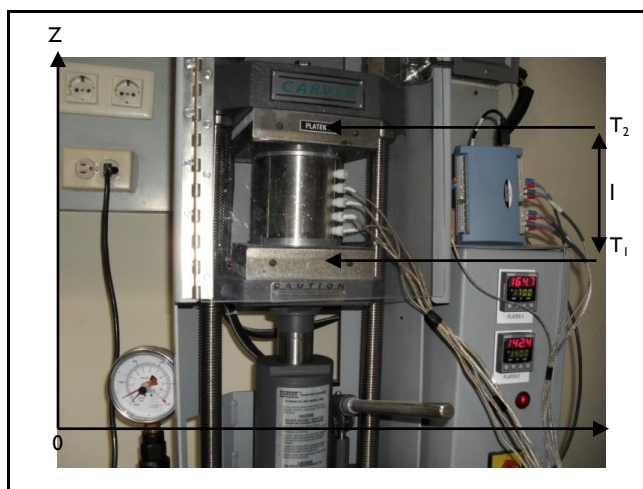
Figure 1. Experimental design for measuring thermal diffusivity. Material with cylindrical geometry, placed between the plates of a press which could be heated to temperatures T_1 and T_2 with T_2 > T_1
