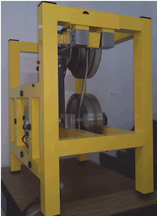
Figure 4. The ABS laboratory setup [11]. Source: Inteco Manual [11].
