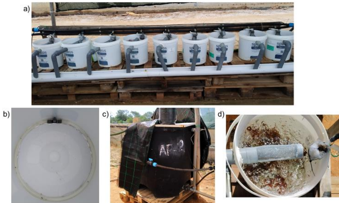
Figure 2.1: System for seaweed cultivation: a) 9 white polyethylene tanks (20 L), continuously supplied with the effluent (Trial 1); b) Seaweed tank in detail, where it is possible to see the tubes placed in the bottom of the tanks and pierced at regular intervals; c) Reservoir tank; d) Seaweed tank in detail, where it is possible to see the inflow water, glass wool filter, and outflow apparatus.
