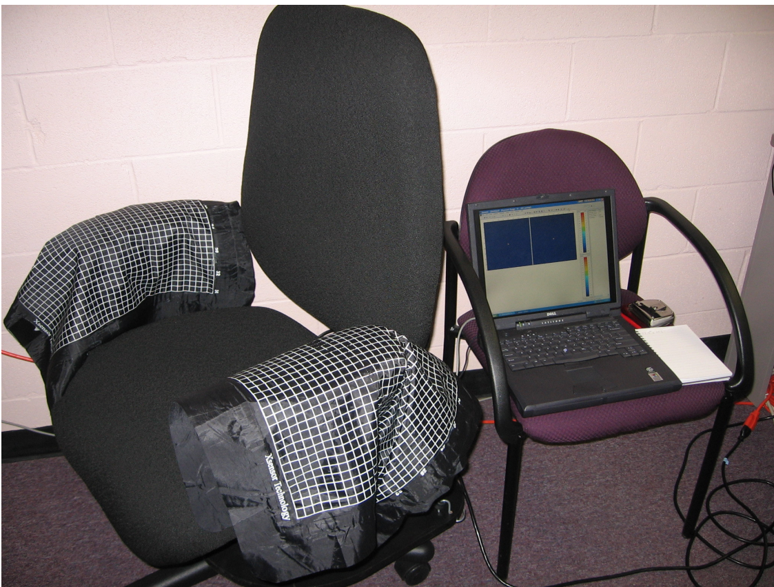
Figure 20 – Arm Test Sensors for Entry/Exit Study
