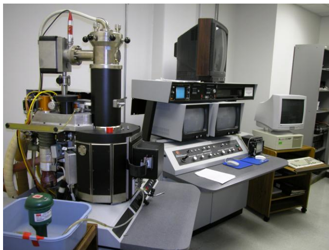
Figure 7. Photograph of the Electron Scanning Environmental Microscope Lab. The microscope and sealed chamber are located on the left.
