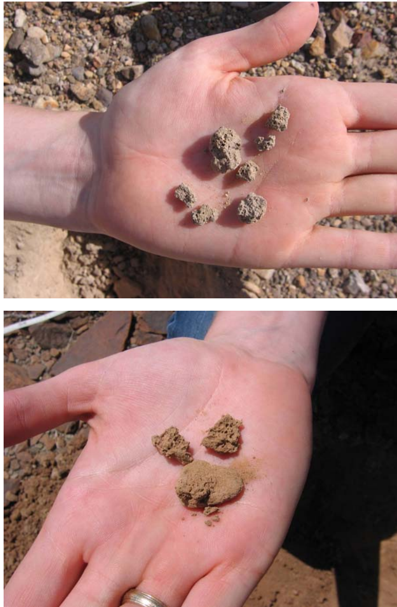
Fig. 19. Soil beneath Study Areas 1 and 2. Examples of well-developed vesicular horizons at Study Area 1 (top) and Study Area 2 (bottom).
