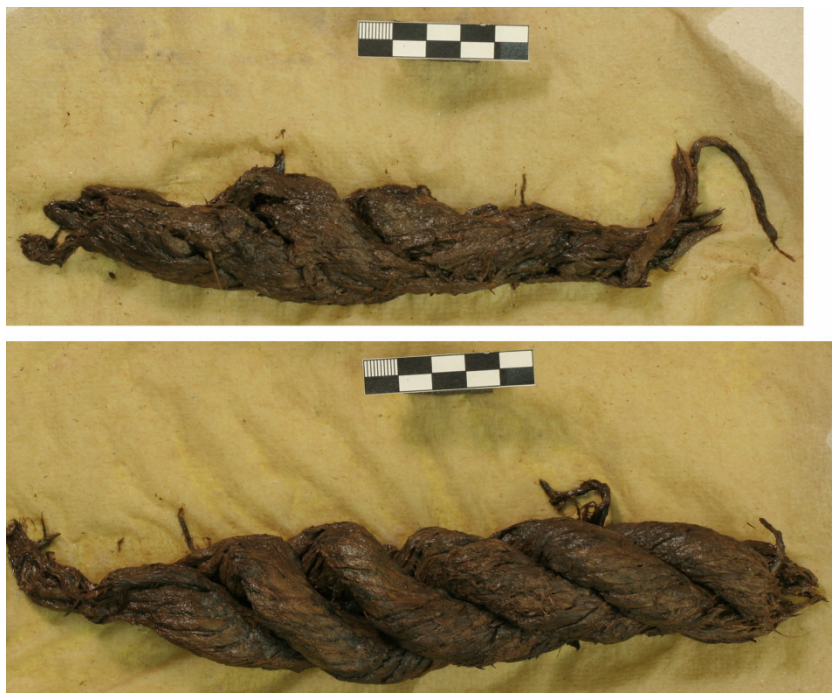
Figure 26. Sample 3 (top) and sample C (bottom), prior to treatment in an aqueous solution of 10 percent Jeffox followed by an aqueous solution of 30 percent PEG 1400. Photo by R. Sasaki.
