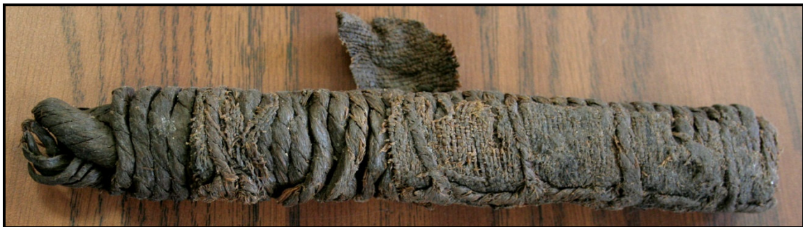
Figure 10. Short segment of rope displaying serving and canvas sail or awning attached with marline hitches. Photo by J. McCaskill.
