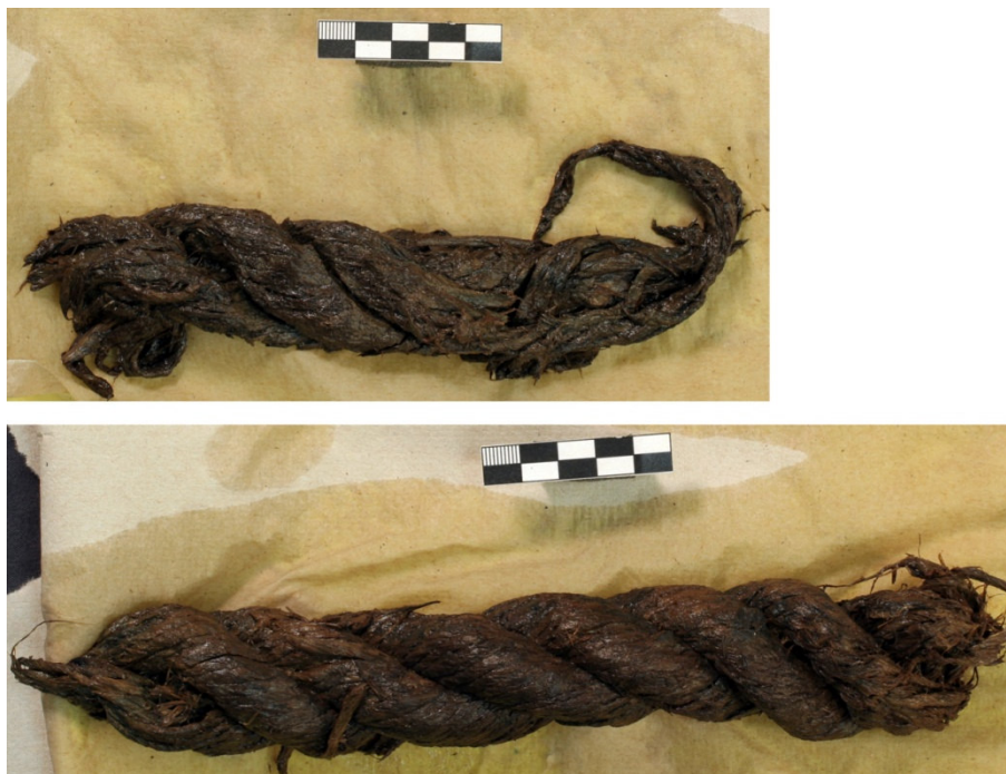
Figure 24. Sample 1 (top) and sample A (bottom), prior to treatment in an aqueous solution of 10 percent Jeffox followed by an aqueous solution of 30 percent PEG 400. Photo by R. Sasaki.
