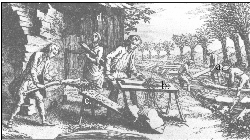
Figure 3. Depiction of the hemp preparation process: (a.) weighing the bundles of hemp for water retting, (b.) scutching the hemp, (c.) drawing the hemp through a set of hackle pins, (d.) the bundles of hemp fibers. Image after H. L. Duhamel du Monceau (1769).
