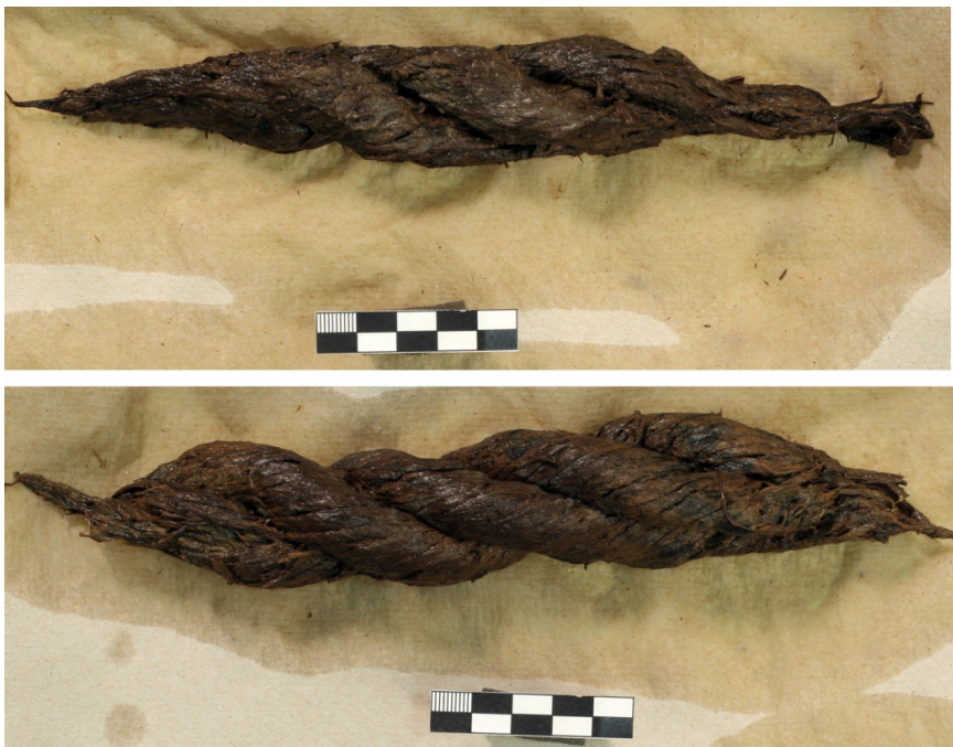
Figure 29. Sample 6 (top) and sample F (bottom), prior to treatment in an aqueous solution of 30 percent PEG 1400. Photo by R. Sasaki.
