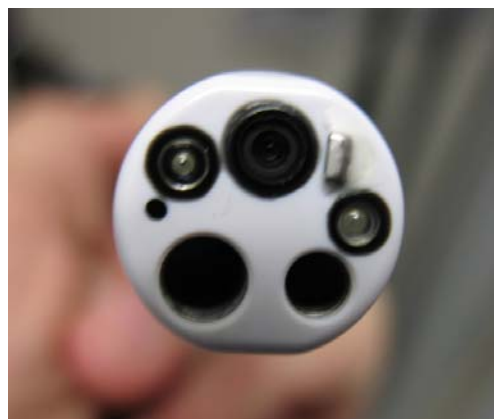
Fig. 29. End view of the GI endoscope.
