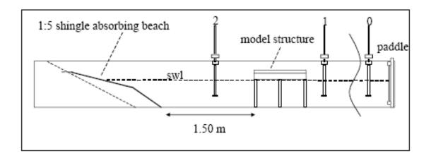
Figure 3.14: Experimental set-up in the wave absorbing flume by Tirindelli et al. (2002)
