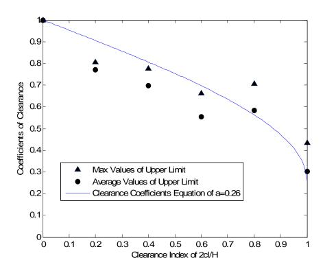
Figure 3.29 Flow3D model maximum uplift wave forces and water clearance coefficients equations and estimate equations
