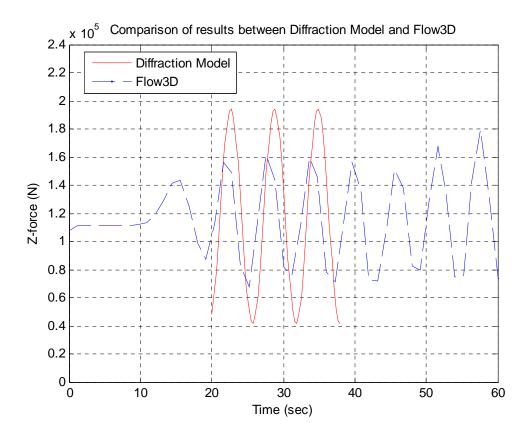
Figure 3.12: Comparison of uplift wave force results between Flow3D and 2D Model
