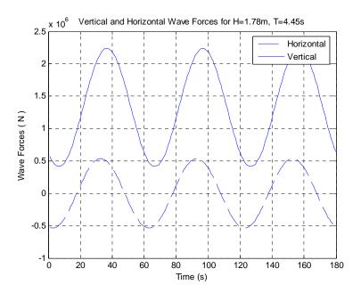
Figure 4.15: Wave force on bridge in reference model with H = 1.78m, T = 4.45s
