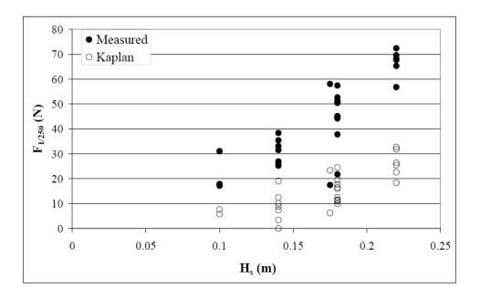
Figure 3.16: Measured uplift wave forces on external deck and Kaplan's predictions (Tirindelli et al., 2002)
