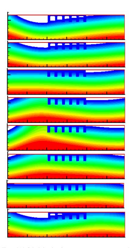
Figure 4.14: Calculation domain pressure contour as waves pass by
