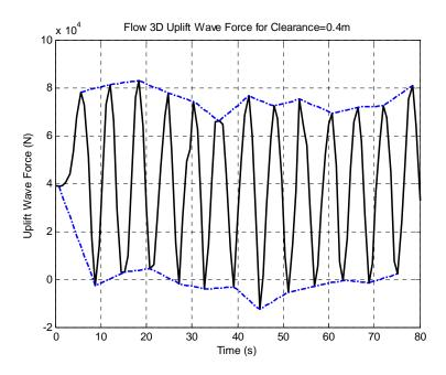
Figure 3.24: Flow3D uplift wave force for H=2m, T=6s, D=6m at clearance=0.4m
