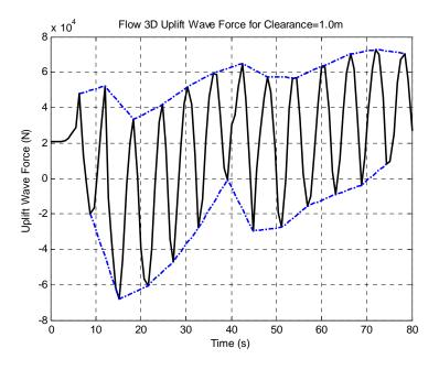
Figure 3.27: Flow3D uplift wave force for H=2m, T=6s, D=6m at clearance=1.0m
