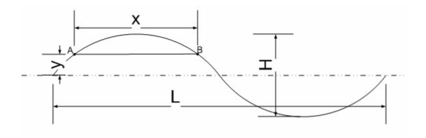
Figure 3.18: Sketch of incoming sinusoidal wave and clearance
