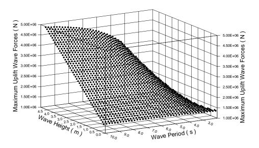
Figure 5.4: 3-D plot of maximum overall uplift wave force (30° degree direction)
