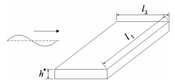
Figure 5.21: A figure showing the relative buoyancy height  $h^*$  (The cube in the figure has the same volume as the model bridge)
