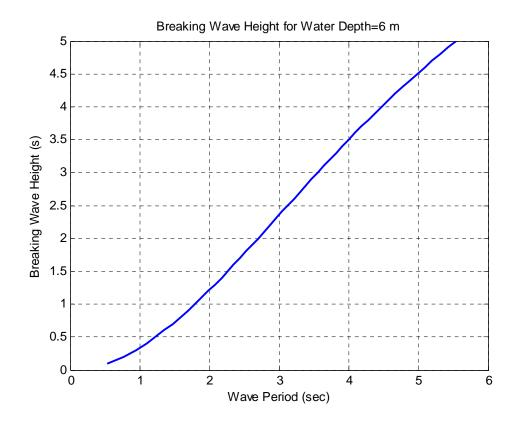
Figure 5.2: Breaking wave height according to wave periods for water depth of 6m
