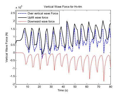
Figure 5.9: Vertical wave forces for H=4m
