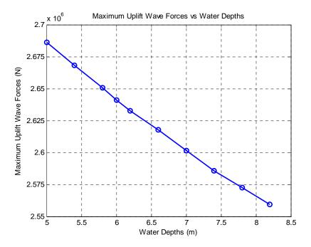
Figure 5.15: Maximum uplift wave forces according to water depth
