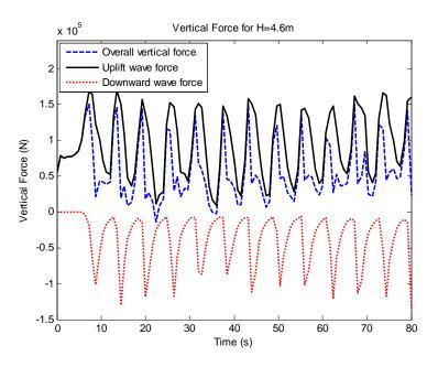
Figure 5.10: Vertical wave forces for H=4.6m
