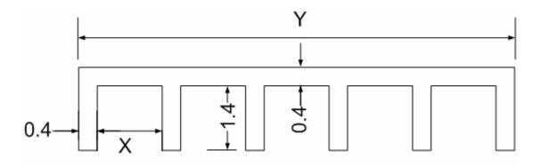
Figure 5.12: Structure component geometry in metric units, x is defined as the distance between the girders and y is defined as the overall width of the bridge deck cross section
