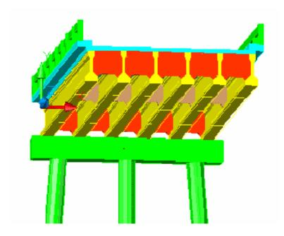
Figure 4.10: Structural geometry of I-10 Bridge over Escambia Bay
