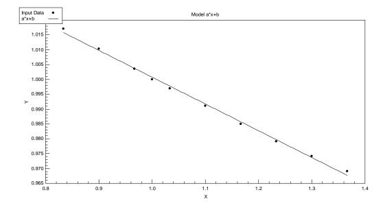
Figure 5.24: Estimation equation for water depth coefficient,  $A_d = ax + b$  where a=-0.090, b=1.091
