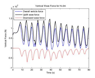
Figure 5.8: Vertical wave forces for H=3m
