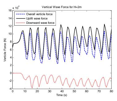
Figure 5.7: Vertical wave forces for H=2m
