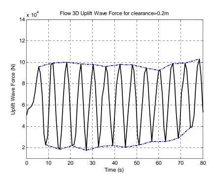
Figure 3.23: Flow3D uplift wave force for H=2m, T=6s, D=6m at clearance=0.2m
