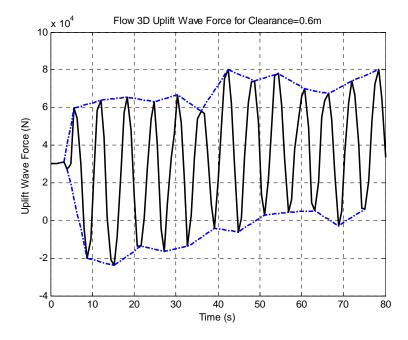
Figure 3.25: Flow3D uplift wave force for H=2m, T=6s, D=6m at clearance=0.6m
