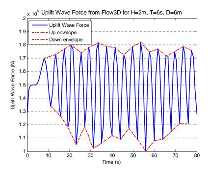
Figure 3.22: Uplift wave forces from Flow3D model for H=2m, T=6s, D=6m
