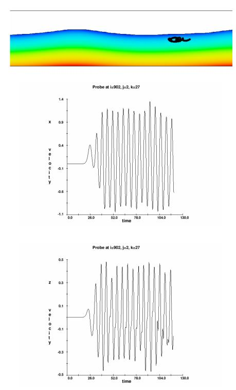
Figure 3.9: Point G particle path and velocities in x and z directions
