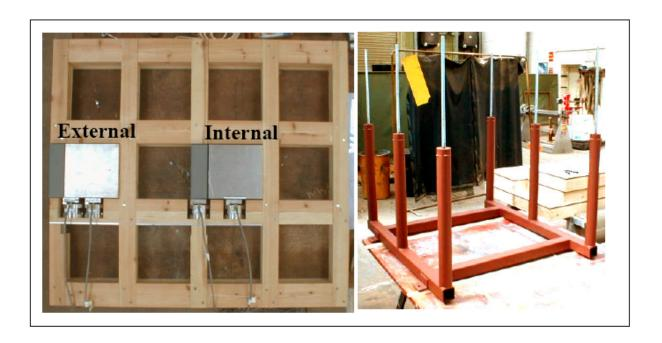
Figure 3.15: Down-standing frame of beams with testing elements and support pile structure (Tirindelli et al., 2002)
