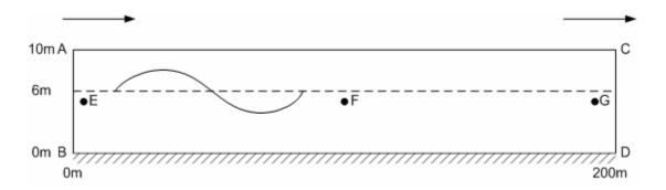
Figure 3.4: Flow3D domain and particle source points
