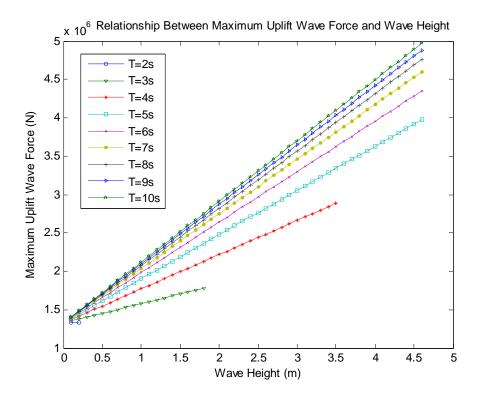
Figure 5.17: Relationship between maximum uplift wave forces and wave heights
