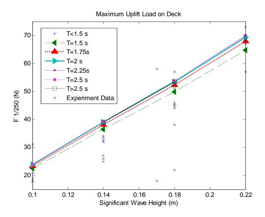
Figure 3.30: Comparison of results from 2D Model and laboratory data from Tirindelli's experiment for the deck
