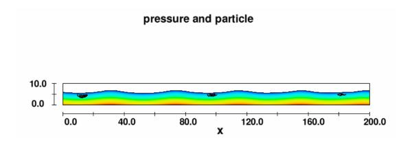
Figure 3.6: The calculation domain and particles moving paths
