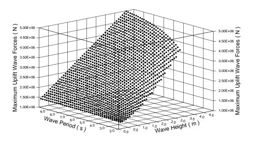
Figure 5.3: 3-D plot of maximum overall uplift wave force (210° degree direction)
