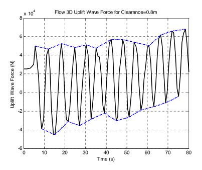
Figure 3.26: Flow3D uplift wave force for H=2m, T=6s, D=6m at clearance=0.8m
