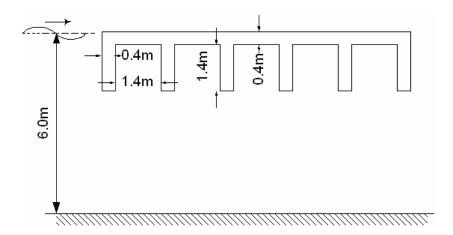
Figure 4.12: Geometry of the bridge deck and girders of reference model
