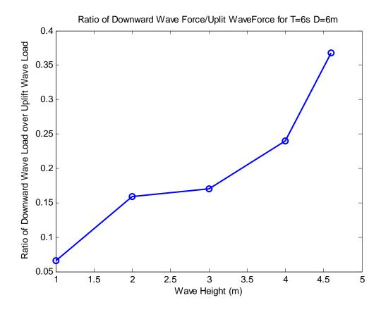
Figure 5.11: Green water load ratio to uplift wave force according to wave heights in the reference model of wave period 6s and water depth 6m.
