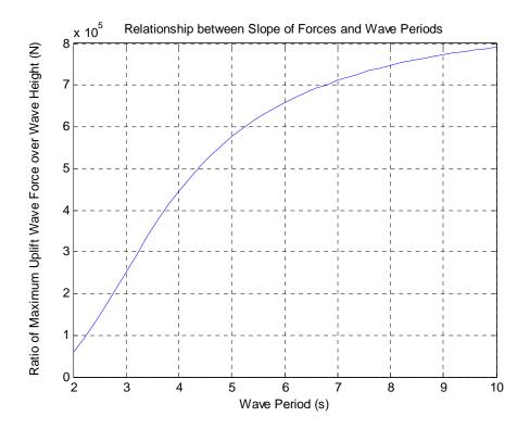
Figure 5.19: Relationship between slope of forces/wave heights and wave periods
