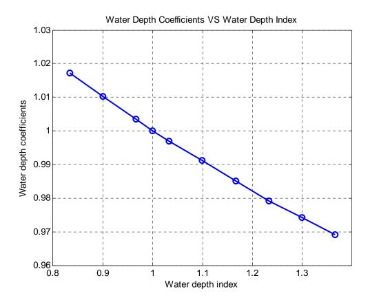
Figure 5.16: Coefficients of water depth for reference model of wave height 2m and wave period 6s
