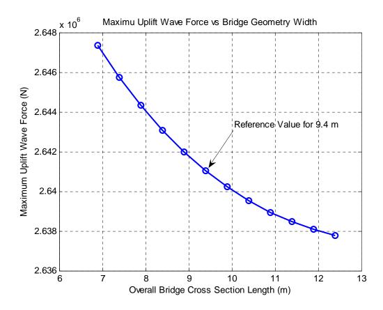
Figure 5.13: Maximum uplift wave forces according to bridge geometry width
