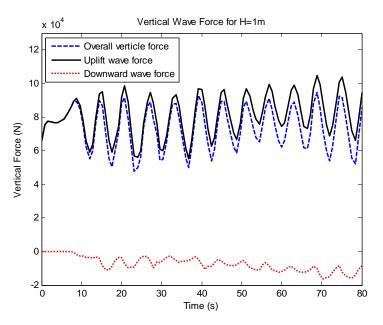
Figure 5.6: Vertical wave forces for H=1m
