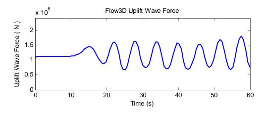
Figure 3.11: Flow3D uplift wave force over simulation time
