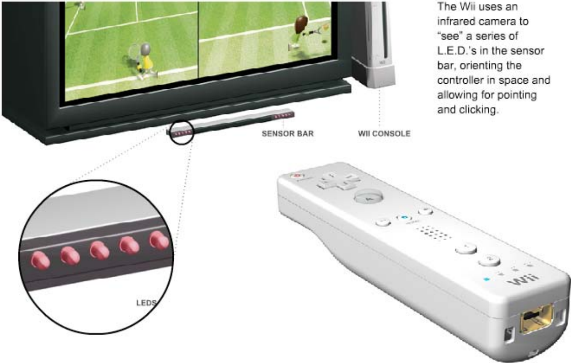
Figure 23. Wiimote pointing bar using the sensor bar [31].
