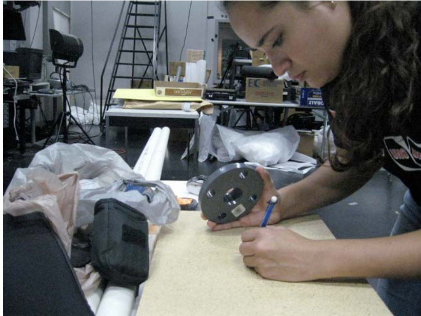
Figure 33. Attaching the flange to the particleboard for the lighting rig base.
