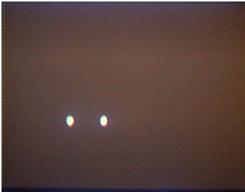
Figure 54. The wiimote's IR camera view of the markers used to calculate x-y screen position.
