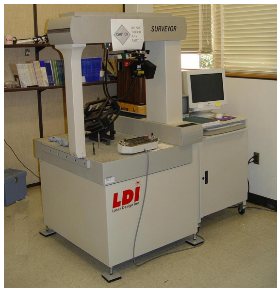
Fig. 30. OCMM: LDI Surveyor DS-2020 with a RPS 150 laser unit
