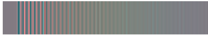
Fig. 87. Voltage profile color pattern for a single-phase to ground fault 20 miles away from bus A - Emboss filter is applied.
