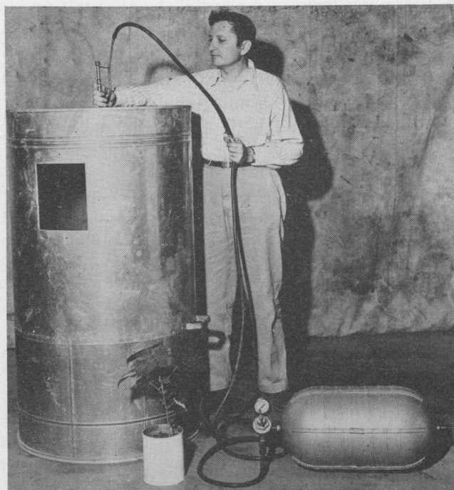
Figure 4. Tower used to apply predetermined dosages of spray emulsions or dusts of insecticides to individual cotton plants.
