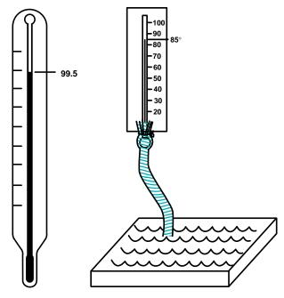
A wet-bulb thermometer is easily made using a dry thermometer. The wet bulb registers a lower temperature than the dry bulb because evaporation cools the thermometer. The wet-bulb reading is an index of relative humidity.
