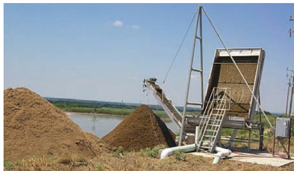
Figure 2. Mechanical solids separation system. Water flows across a sloped screen that collects the solids. The solids then fall to the bottom and are collected by an auger and stacked using the flighted-conveyor separator.
