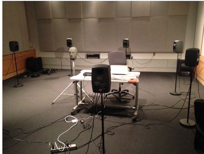
Figure 1: Loudspeakers and dummy-head microphone layout inside the laboratory.
