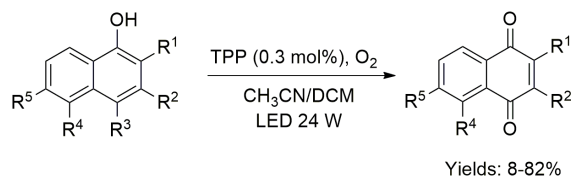
Figure 25 - Photocatalyzed photooxygenation of hydroquinones under flow conditions reported by de Oliveira and McQuade (de Oliveira et al. 2016).
