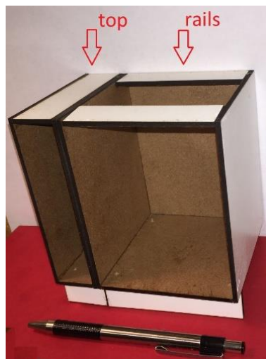
Figure 79 - Scaled cabinet fabricated in laser CNC machine
