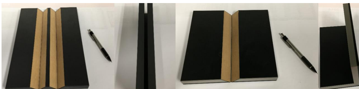
Figure 58 – Folding by mitred-cut as a digital fabrication technique
