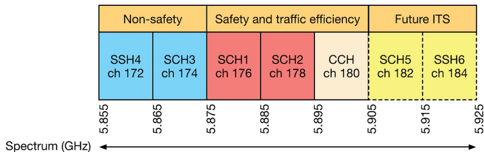
Figure 2.7: Multichannel operation in VANETs according to the IEEE 802.11p European standard (Source [51]).
