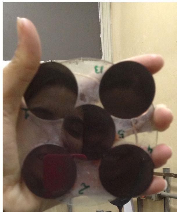
Figure 3. Blocking having 5 samples during polishing process (flat).
